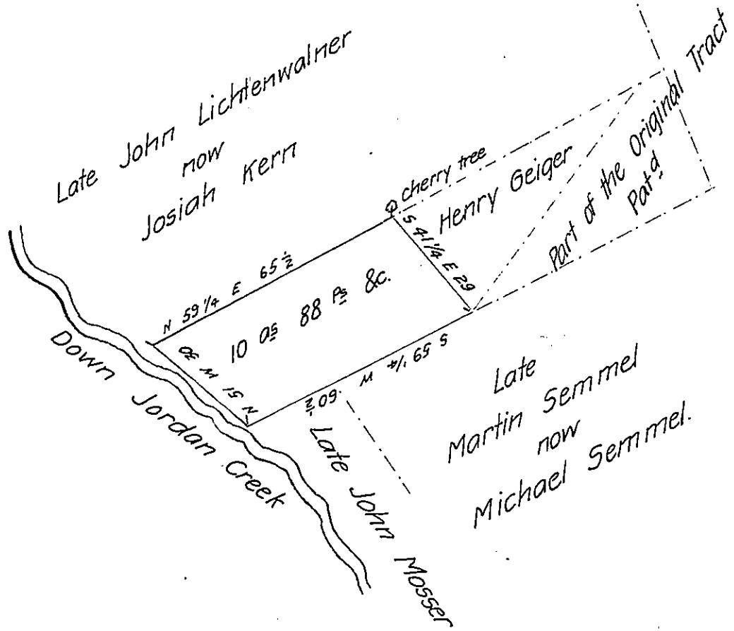
Draft of a tract of land situate in Whitehall township Lehigh County Containing 10 ac 88 ps and allowance of six per cent for roads &c. Surveyed for Josiah Kern the 4<sup>th</sup> day of April A.D. 1873 being a part of a larger tract of 24 ac 23 ps & allowance Originally suyed in pu-
